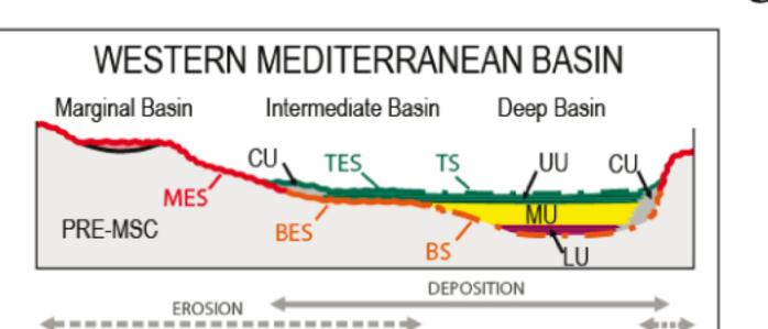
Figure 5. Idealized schematic cross section for the western Mediterranean basin, illustrating the geometric organization of the MSC seismic markers in the (Lofi et al., 2011a and 2011b). MSC: Messinian Salinity Crisis, MES: Margin Erosion Surface, BES: Bottom Erosion Surface, BS: Bottom Surface, TES: Top Erosion Surface, TS: Top Surface, UU: Upper Unit, MU: Mobile Unit, Lower Unit, CU: Complex Unit (Lofi et al., 2011).
